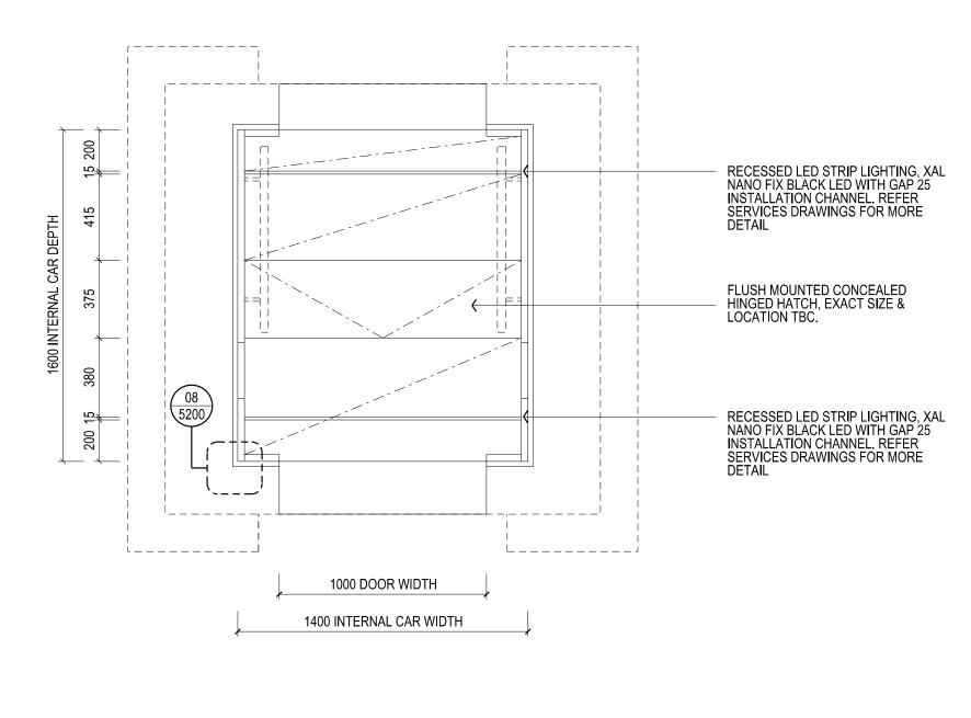
06 REFLECTED CEILING PLAN - LIFT CAR 04, 05 - SCALE 1:20
